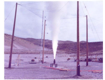
Measurements of the charging of solid rocket engines exposed to static electric fields gives insight into charge transport in rocket plumes and lightning hazards to launch vehicles.
