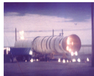
Full scale lightning testing of space shuttle solid rocket booster engines.
