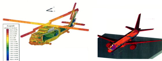
Aircraft models can be derived from paper drawings or CAD files.
