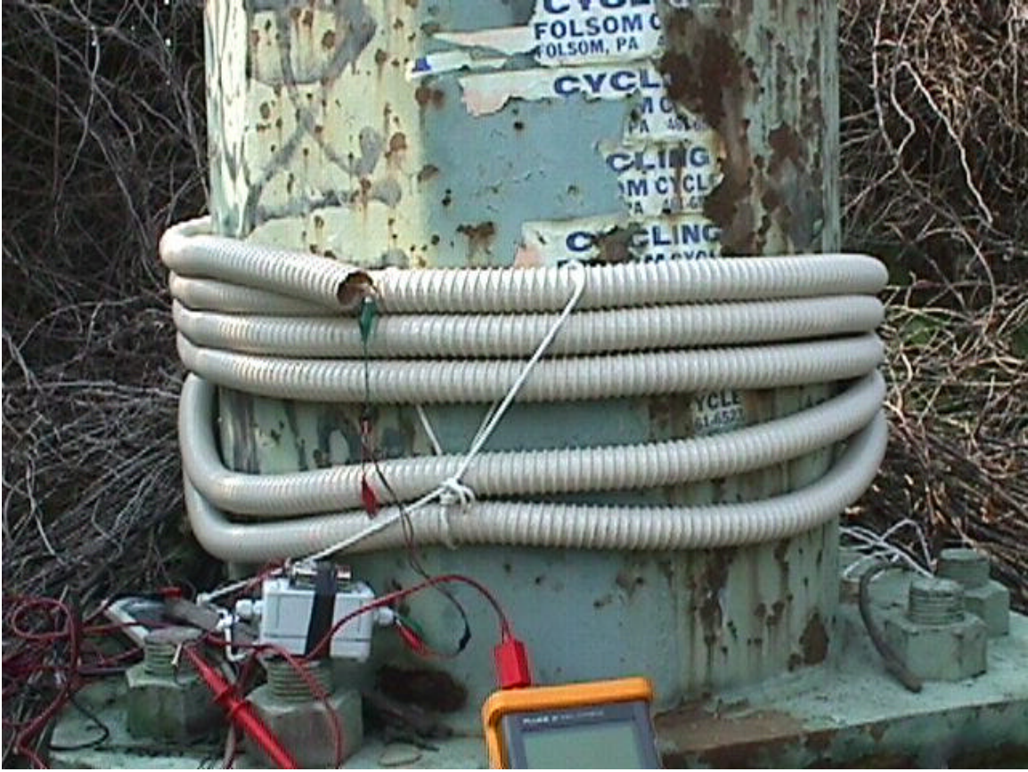
A novel approach for measurement of leakage currents in large steel transmission line towers
