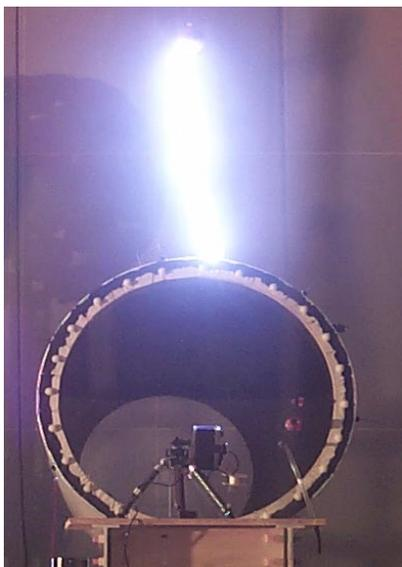
Figure 6. Lightning Leader Voltage Test on the 1:65 scale cylinder
