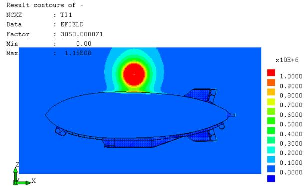
Figure 10. Field Distribution on the Airship Due a Leader 25 Meters above
