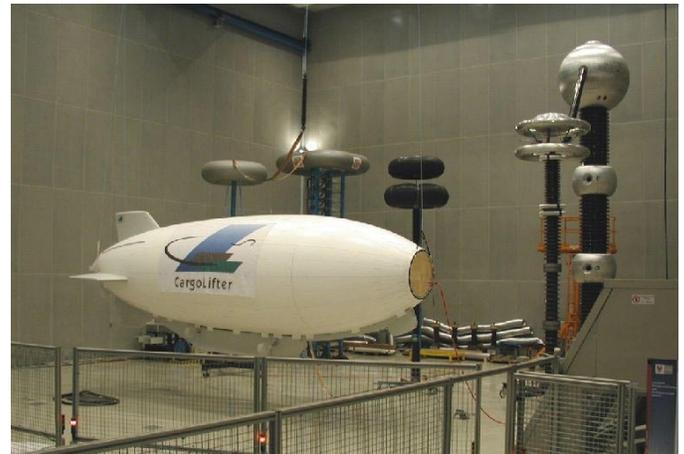
Figure 7. 1/25 Scale Model of CL 160 in BTU HV Laboratory
