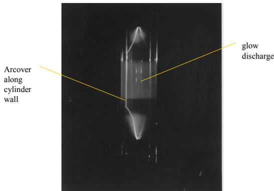
Figure 4. Helium Breakdown in Cylinder
