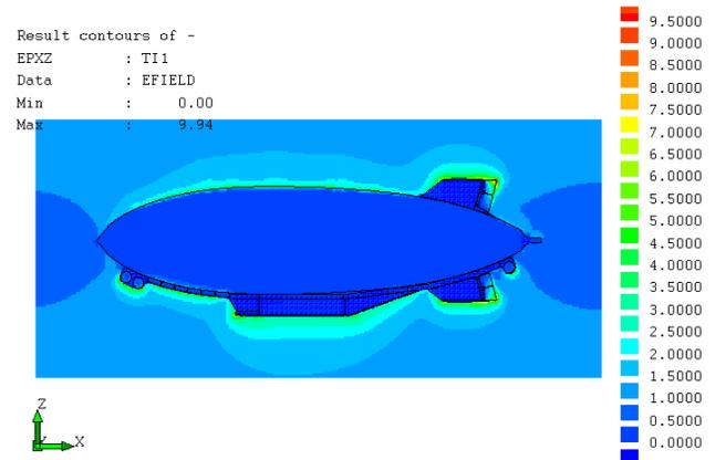
Figure 8. Typical Example of Airship Field Enhancement Factors for a Vertical Uniform Incident Static Electric Field for Triggered Lightning Evaluation
